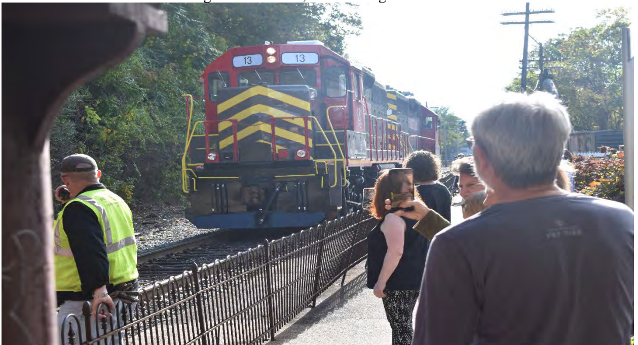
BB GP-40-2 coming to hook onto the end of the train to pull the train back to Goshen, VA
