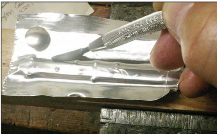
Both photos-Burnishing tool on foil for detail
