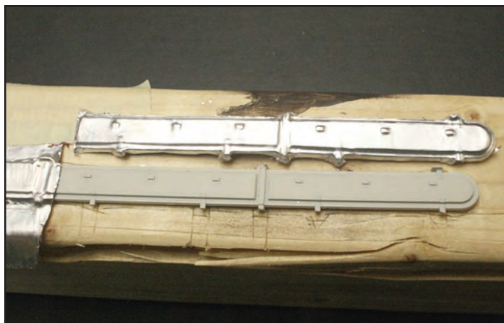
Plastic covered hopper hatch with replica casting on wood base
