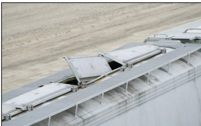
Damaged hatches are common sights at Galesburg Yard's RIP Track
