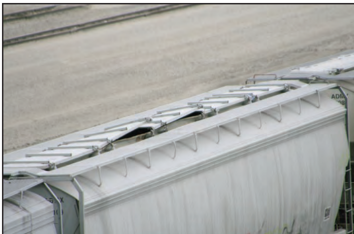
Damaged hatches are common sights at Galesburg Yard's RIP Track
