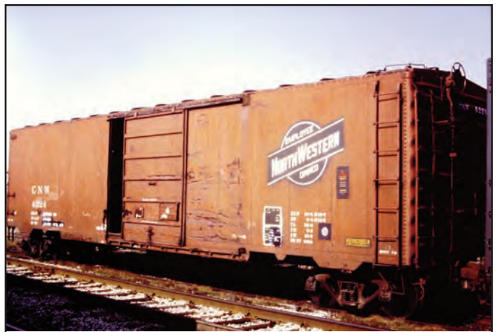
Top photo is a prototype shot showing the deep scratches a boxcar door leaves in the sides of the car.
