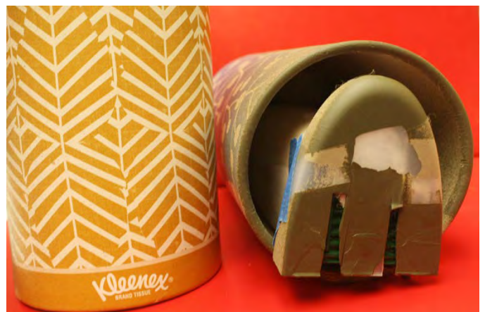
Photos 7 to the left and 8 above show a boxcar with the dental floss container mask at the end. The paper wrapped around the car near the end protects it from overspray. The entire car is placed inside a round Kleenex tissue dispenser to protect the unmasked part of the car from any overspray.
