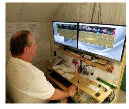
Above, Greg Bedlek is at the GNP's dispatcher's desk. The layout's fully functional—including route locking— and fully displayed CTC machine is shown on two large computer screens. The layout is dispatched using this computer system. As one of the country's top computer programmers, Greg wrote all of the software that runs his CTC machine which, in turn, runs the railroad. Greg's software is similar to Dr. Bruce Chubb's.
