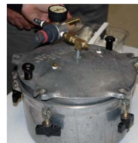
Home made pressure pot from a second hand pressure cooker.
