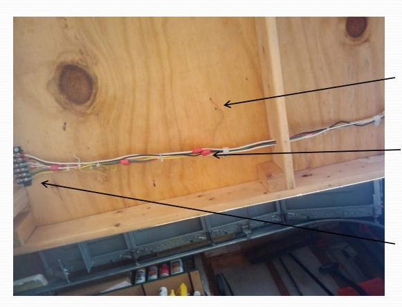
Each section of track has a pair of feeder wires that drop down to the main power bus.
